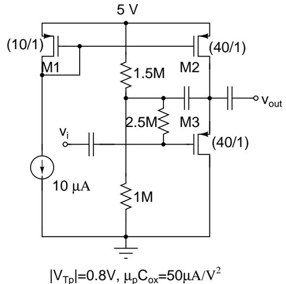
$$|V_{Tp}|=0.8V, \mu_p C_{ox}=50\mu A/V^2$$
