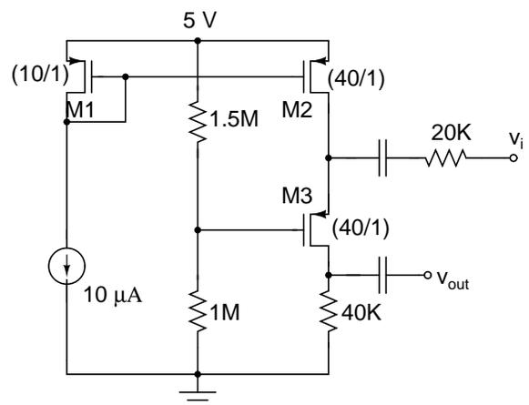
$$|V_{Tp}|=0.8V, \mu_p C_{ox}=50\mu A/V^2$$
