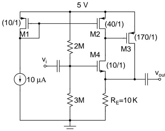
$$V_{Tn}=0.7V, \mu_n C_{ox}=200\mu A/V^2$$
