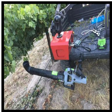
Figure 1: Picture of camera rig and leaf blower in vineyard row.
